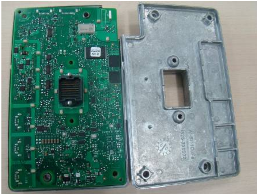
Figure 1: EUT – Internal view 1: Top side
