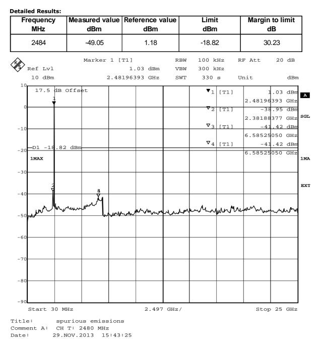
Test: 15c.6; Frequency = 2480, Mode = BT transmit using 2 Mbps with PI/4 DQPSK modulation, Method = radiated
