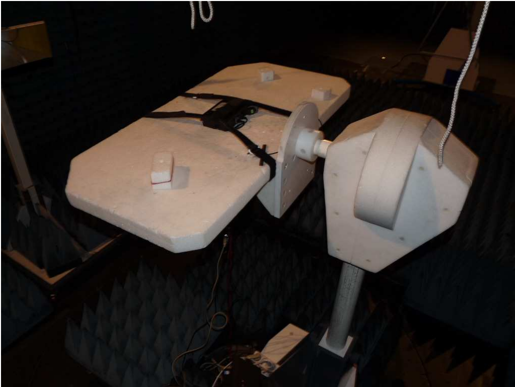
Photo 2: Test setup for radiated measurements (above 1 GHz), FCC 15.247
