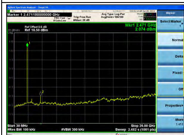
11b-Out Of Band Emission-High
