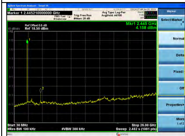
11b-Out Of Band Emission-Mid
