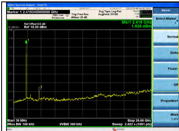
11b-Out Of Band Emission-Low
