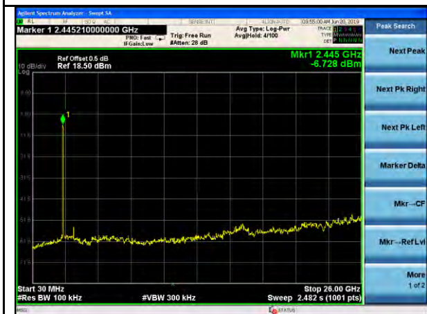
11n 20MHz-Out Of Band Emission-High
