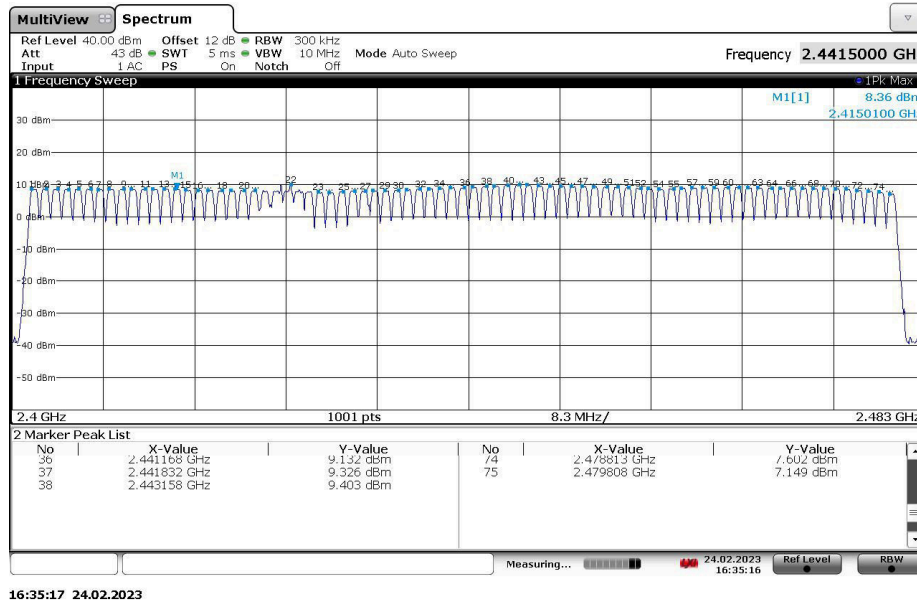
Figure 9: Example Measured Number of Hopping Channels.
