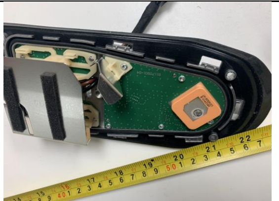
External rooftop antenna#1 - Side View
