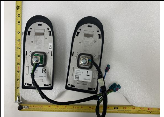
External rooftop antenna - Bottom View
