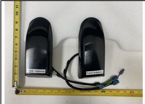
External rooftop antenna - Top View
