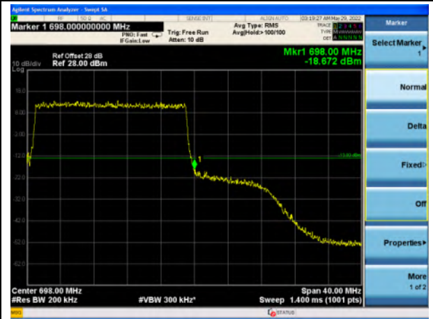
Band 71_16-QAM_20M_High_Full RB Config
