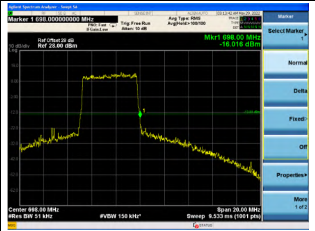
Band 71_16-QAM_5M_High_Full RB Config
