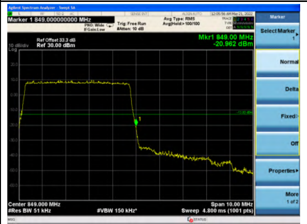
Band 5_16-QAM_5M_High_Full RB Config
