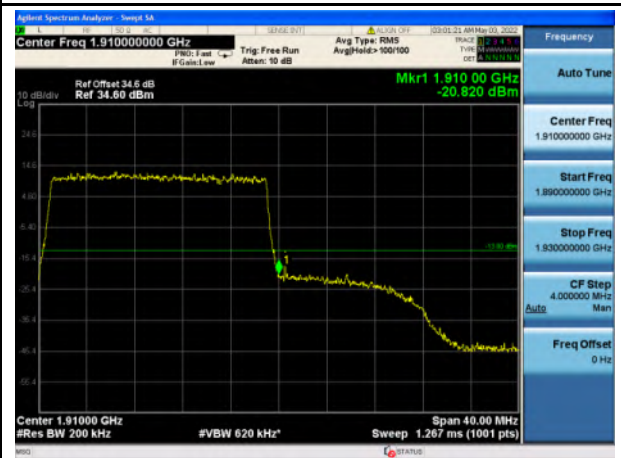
Band 2_16-QAM_20M_High_Full RB Config
