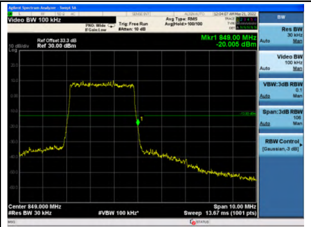
Band 5_16-QAM_3M_High_Full RB Config
