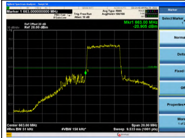
Band 71_16-QAM_5M_Low_Full RB Config
