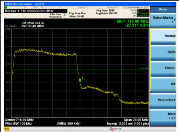
Band 12_16-QAM_10M_High_Full RB Config
