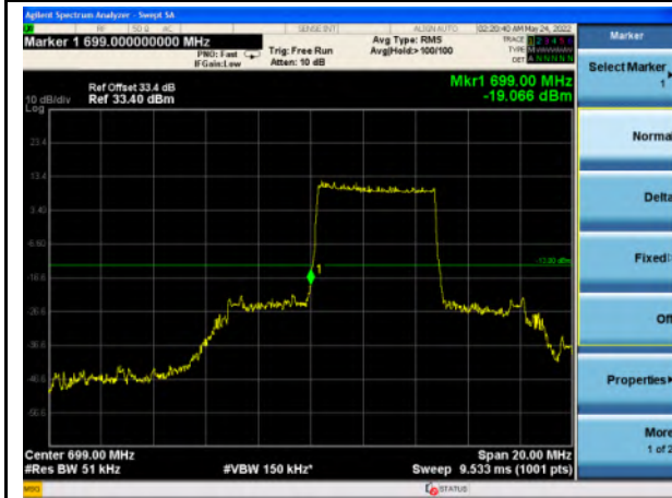
Band 12_QPSK_5M_Low_Full RB Config
