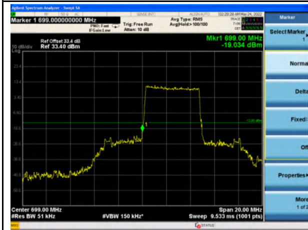
Band 12_16-QAM_5M_Low_Full RB Config
