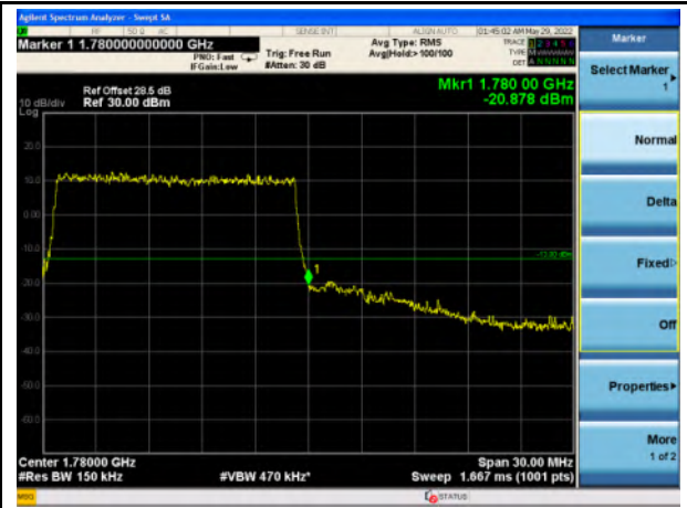
Band 66_16-QAM_15M_High_Full RB Config
