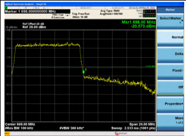
Band 71_16-QAM_10M_High_Full RB Config
