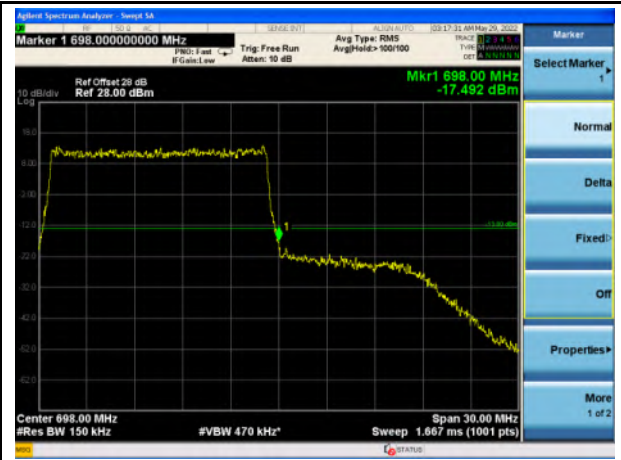
Band 71_16-QAM_15M_High_Full RB Config
