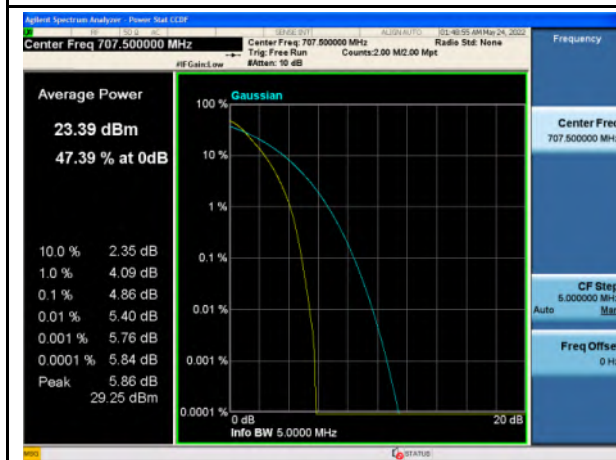
Band 12_QPSK_5M_Mid_Full RB Config
