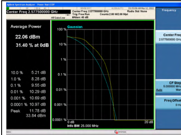
Band 38_QPSK_15M_Low_Full RB Config
