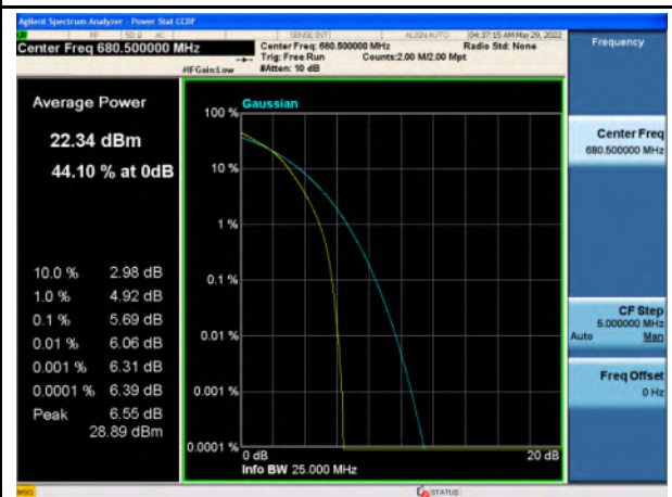
Band 71_16-QAM_15M_Mid_Full RB Config
