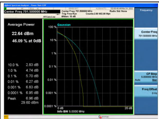
Band 12_16-QAM_5M_Low_Full RB Config
