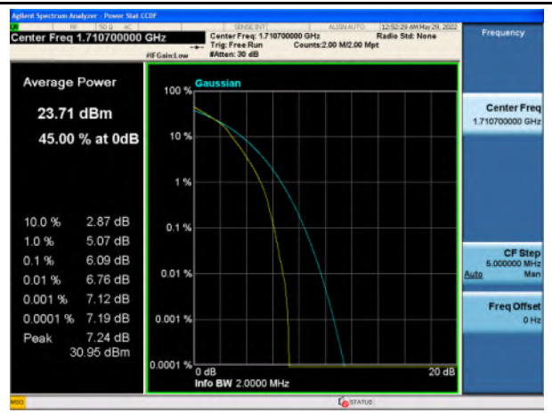
Band 66_16-QAM_1.4M_Low_Full RB Config
