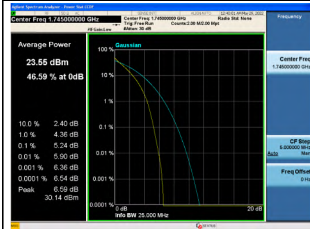
Band 66_QPSK_20M_Mid_Full RB Config
