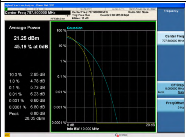
Band 12_16-QAM_10M_Mid_Full RB Config
