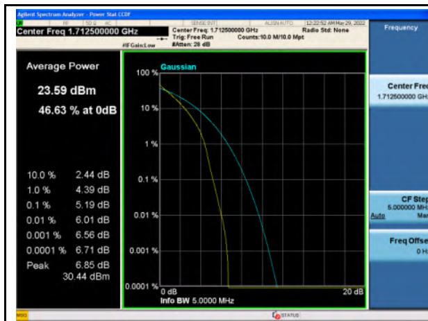
Band 66_QPSK_5M_Low_Full RB Config
