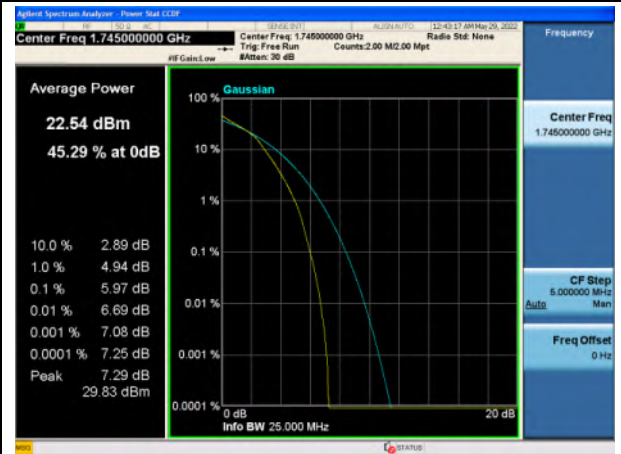
Band 66_16-QAM_20M_Mid_Full RB Config
