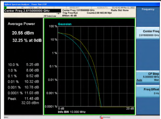
Band 38_16-QAM_10M_High_Full RB Config
