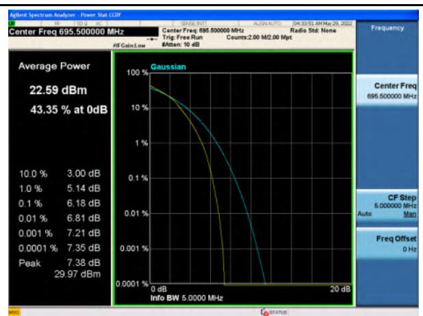
Band 71_16-QAM_5M_High_Full RB Config
