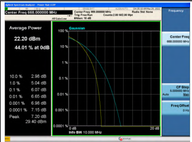
Band 71_16-QAM_10M_Low_Full RB Config
