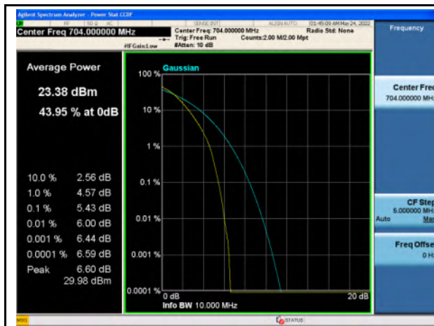
Band 12_QPSK_10M_Low_Full RB Config
