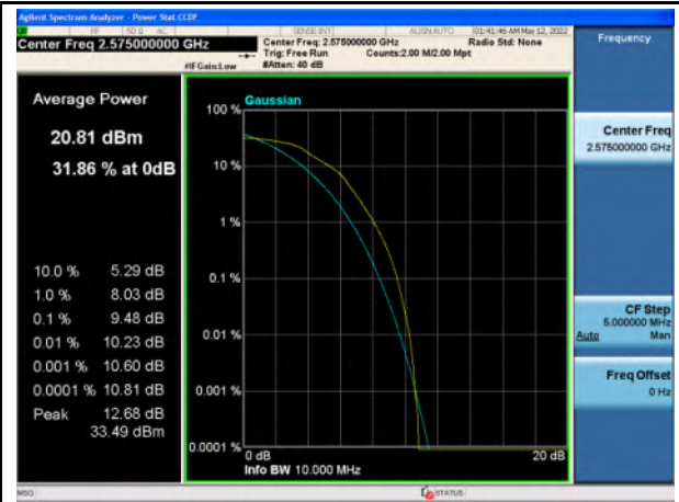
Band 38_16-QAM_10M_Low_Full RB Config
