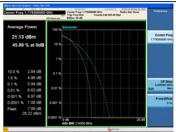
Band 66_16-QAM_1.4M_High_Full RB Config
