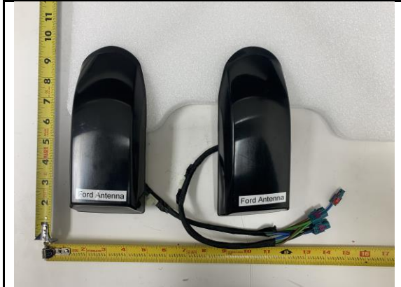
External rooftop antenna - Top View
