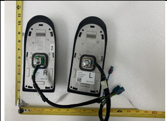
External rooftop antenna - Bottom View
