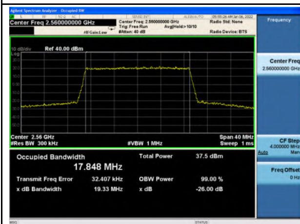
Band 7_QPSK_20M_High_Full RB Config
