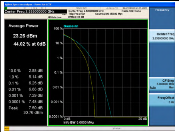
Band 7_16-QAM_5M_Mid_Full RB Config
