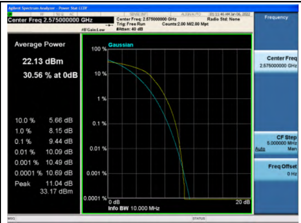
Band 38_16-QAM_10M_Low_Full RB Config
