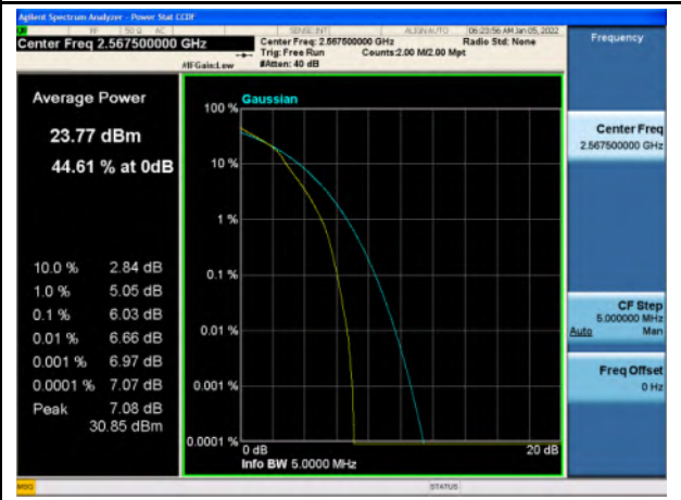
Band 7_16-QAM_5M_High_Full RB Config
