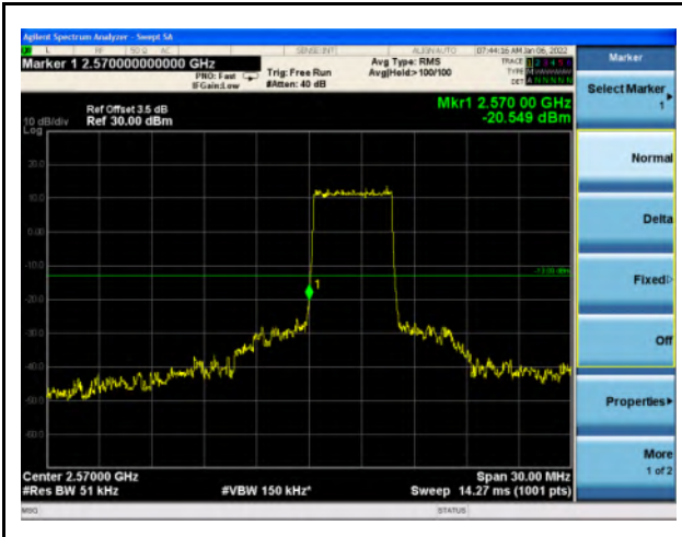
Band 38_QPSK_5M_Low_Full RB Config
