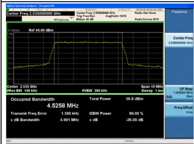
Band 7_QPSK_5M_Mid_Full RB Config
