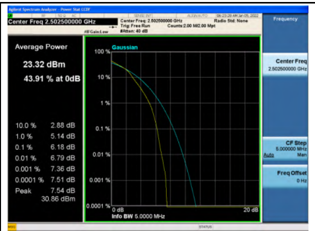
Band 7_16-QAM_5M_Low_Full RB Config
