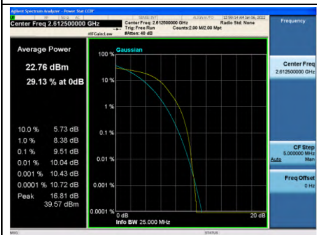
Band 38_QPSK_15M_High_Full RB Config
