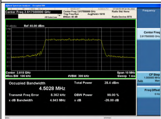
Band 38_QPSK_5M_High_Full RB Config
