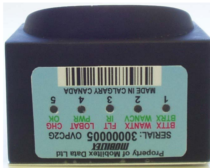
Figure 5 - OVPC Front View - LED Indicators
