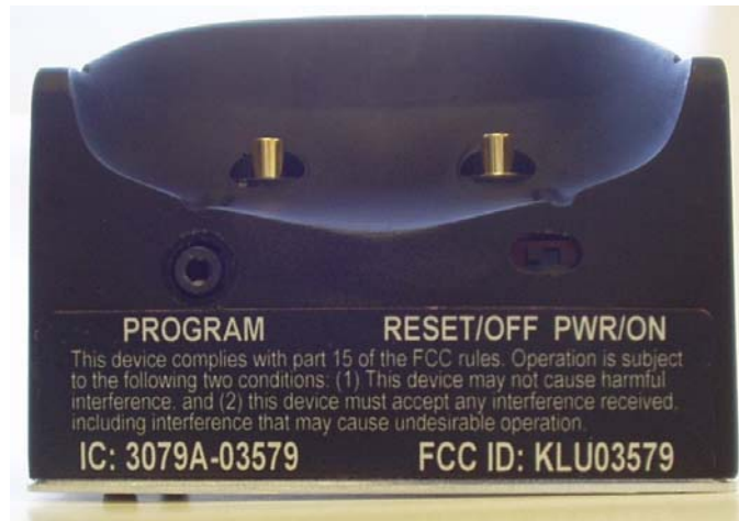
Figure 4 - OVPC2G Rear View - Maintenance Port and Switch
