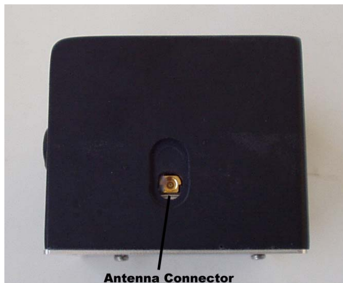
Figure 6 - OVPC2G Side View - Antenna Port
