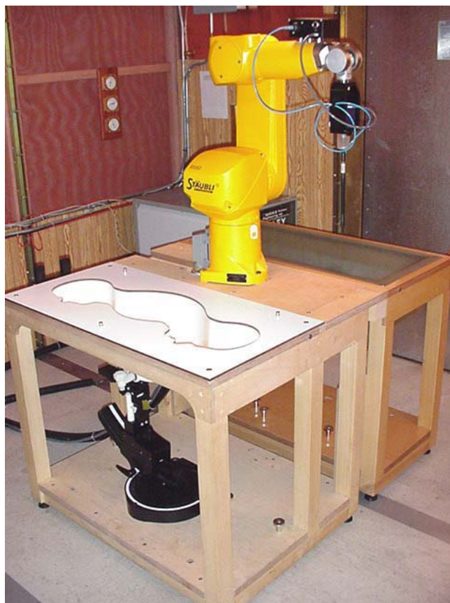
DASY4 SAR Measurement System with SAM phantom
