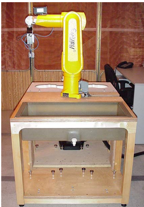
DASY4 SAR Measurement System with planar phantom
