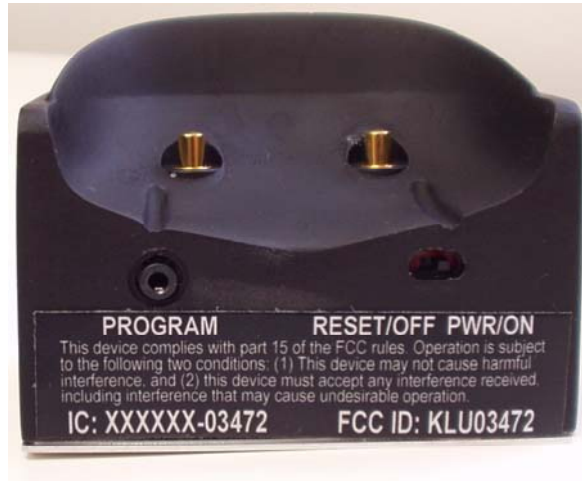
Figure 4 - OVPC2 Rear View - Maintenance Port and Switch
