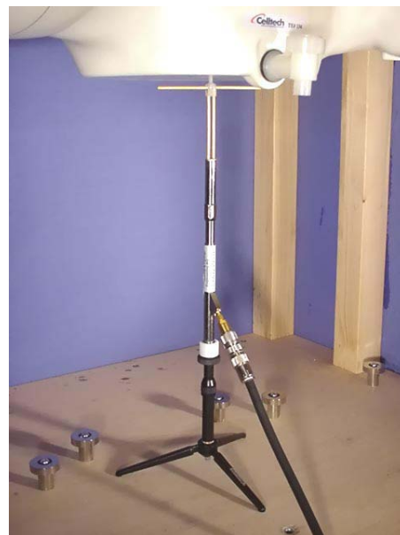
900MHz System Check Setup
