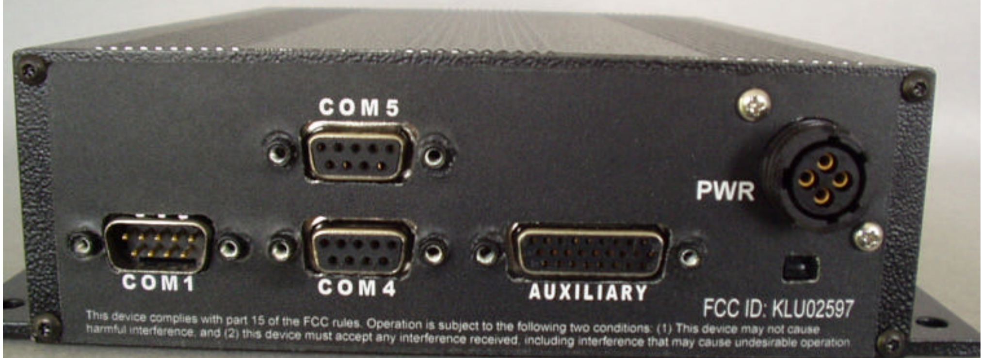
Rear Panel View of OVC3 Showing Location of FCC Label
