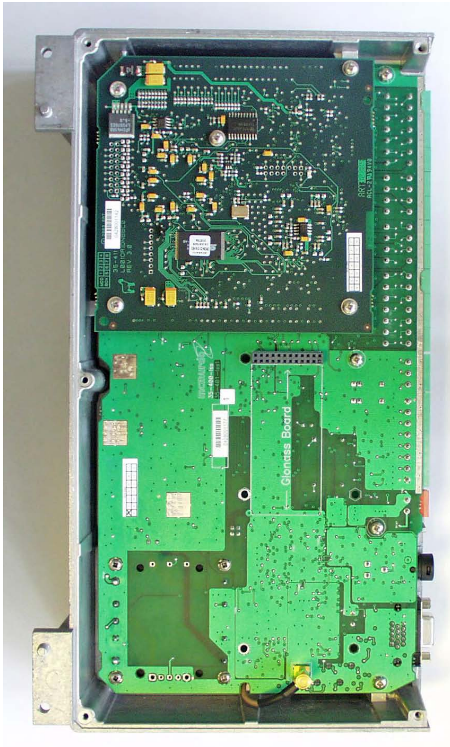
Photograph 6: Opened enclosure, logic board and connection board side
