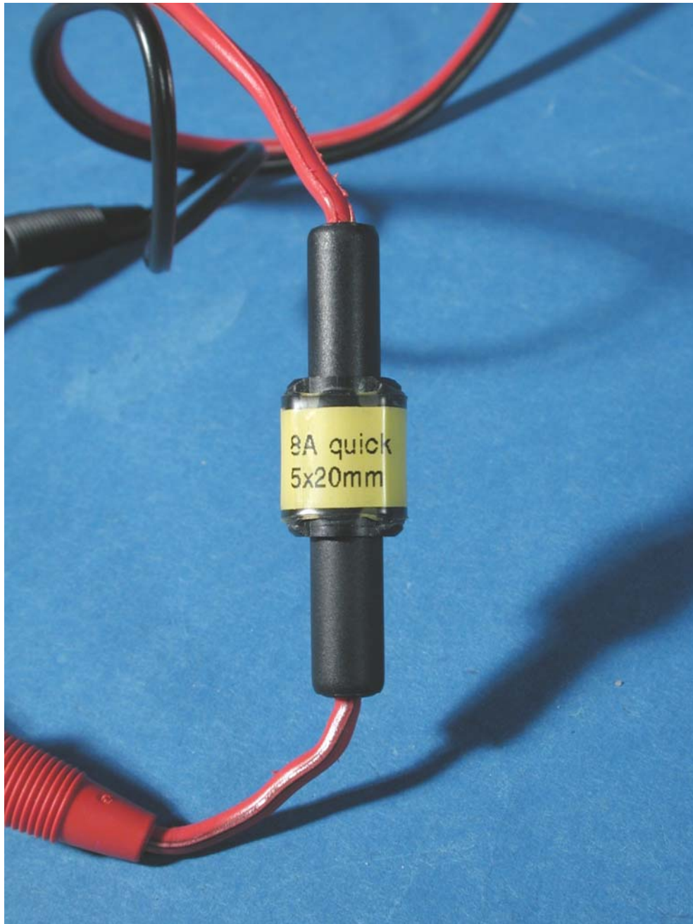
Photograph 6: - Modification, marking added on fuseholder
