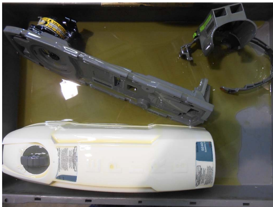
EUT post oil immersion
