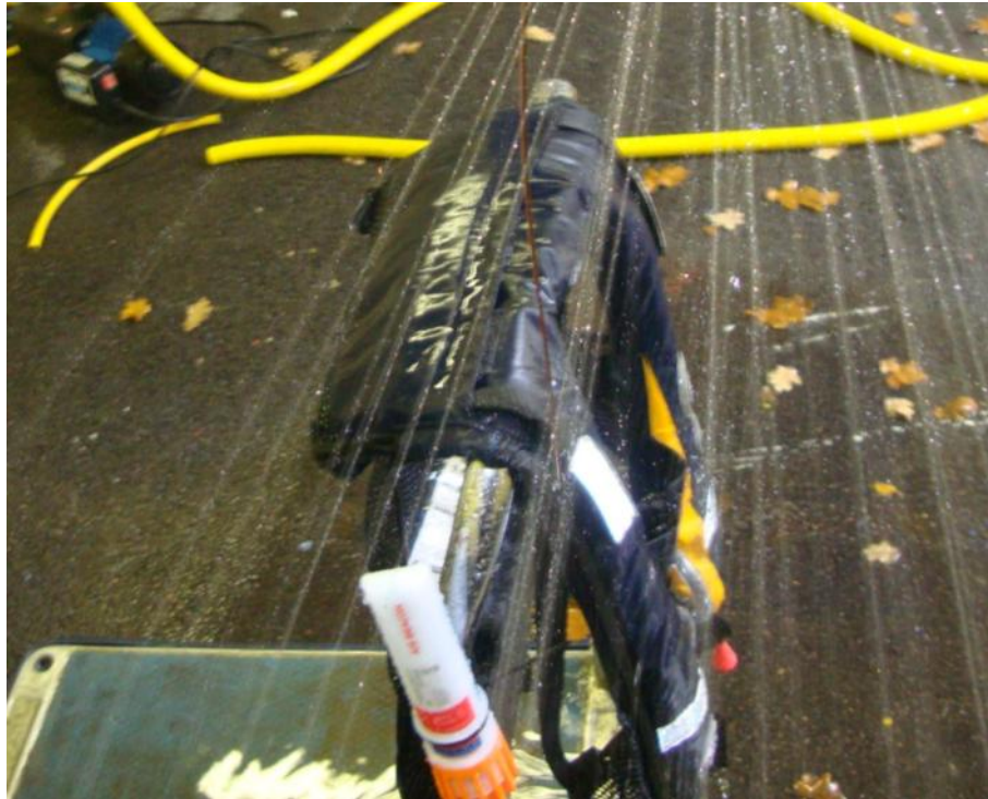
Test Set-up – Rain/Spray Non-Activation (Z501 installed in lifejacket and Z502 standalone)
