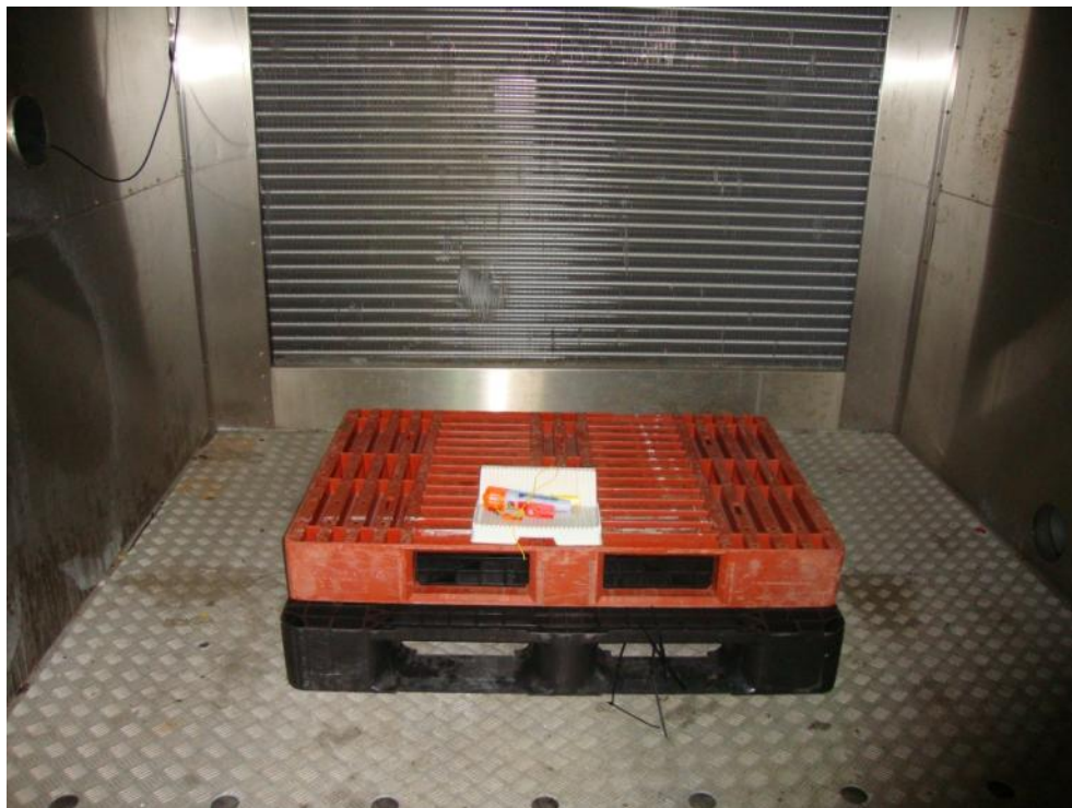
Test Set-up – Thermal Shock (EUT pre-conditioning)
