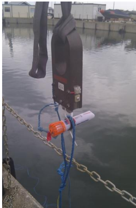
Test Set-up – Drop into Water Z501 installed in lifejacket and being hoisted by crane
