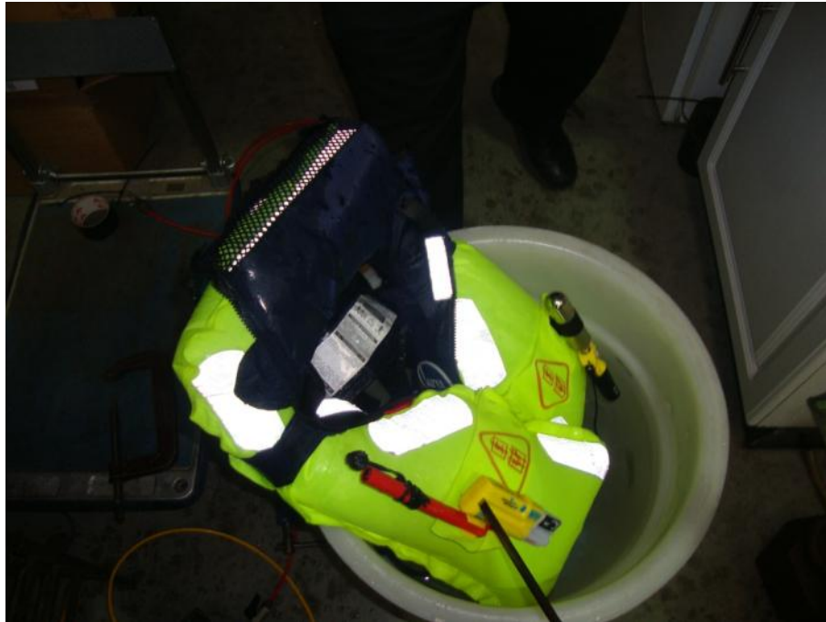
Test Set-up – Z501 Water Activation
