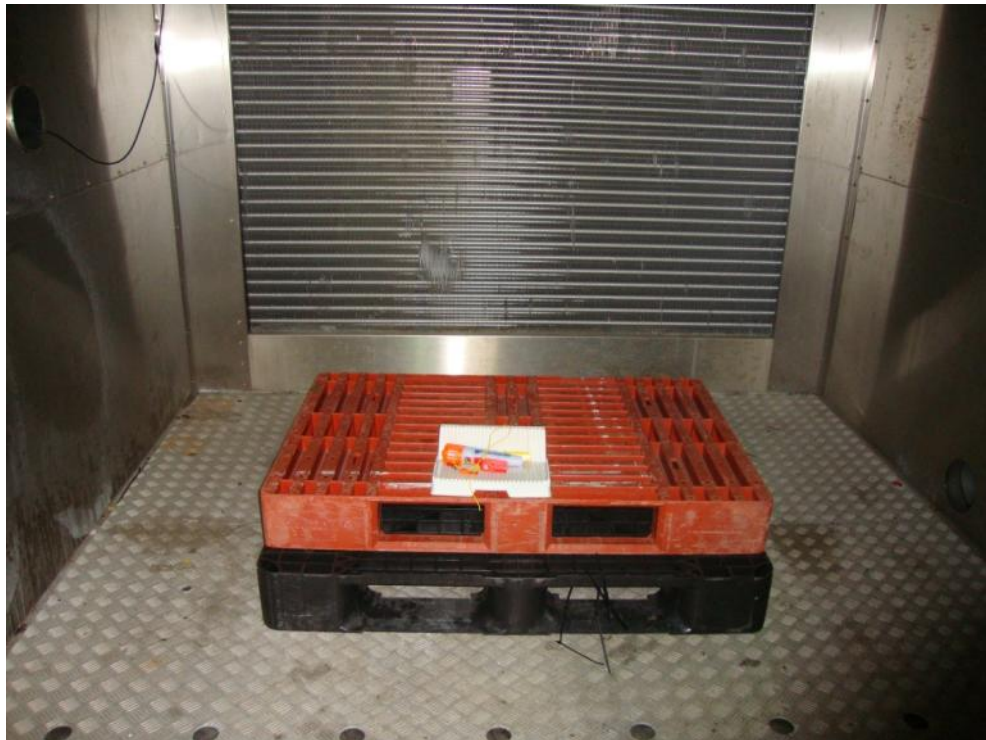
Test Set-up – Thermal Shock (EUT pre-conditioning)
