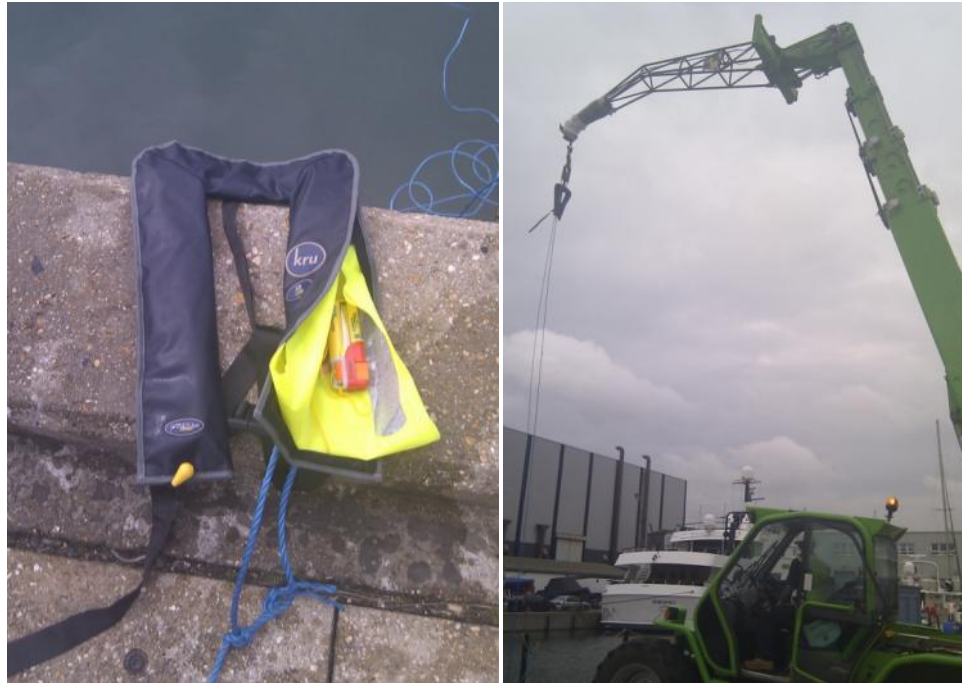
Test Set-up – Drop into Water Z501 installed in lifejacket and being hoisted by crane
