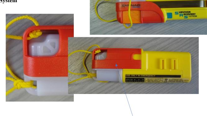
The antenna is folded and retained under the red Activation Cap
