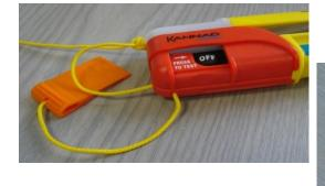
DEPLOYED - the red Activation Cap has been pulled causing the antenna to deploy and the beacon to activate
