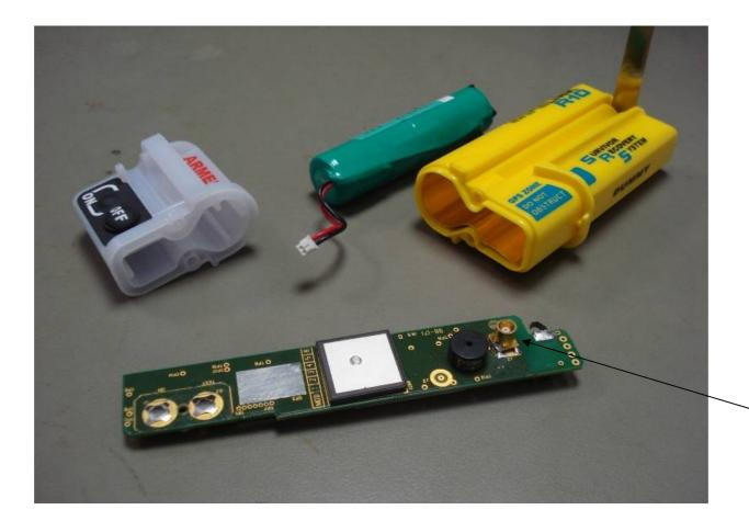
This is a 50 ohm test socket not fitted on production units
