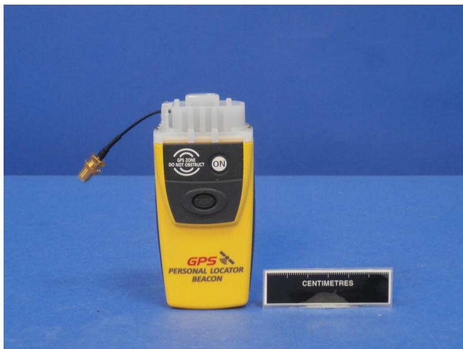
Modified Test Sample - 50Ohm conducted output
