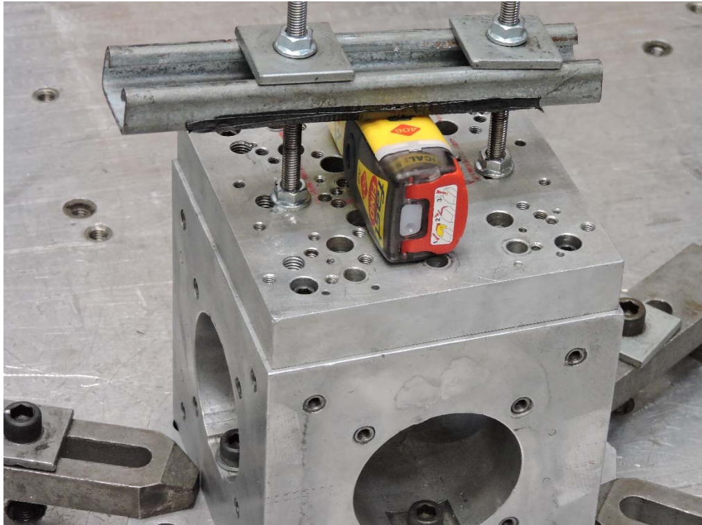
Figure 2.6.3 Shock Test Set-up – Z Axis (Positive)
