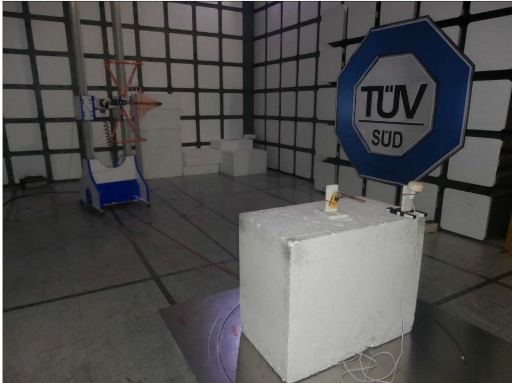
Figure 8 - Test Setup - 30MHz to 2GHz
