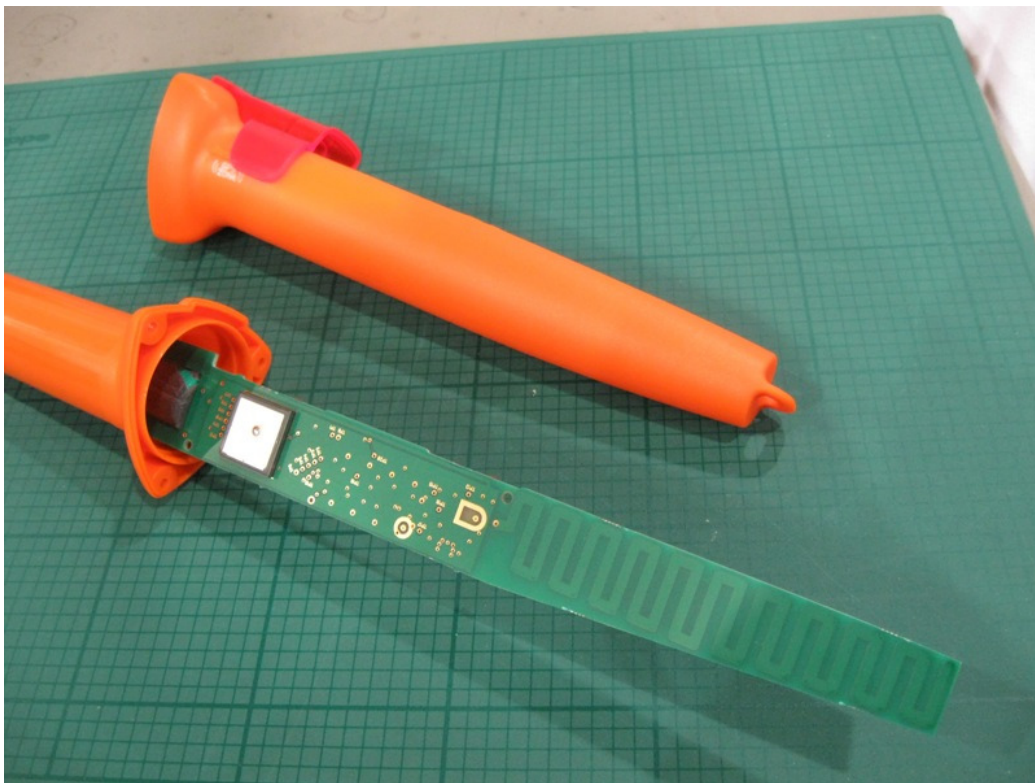
McMurdo Smartfind S5 - reverse side with GPS patch antenna
