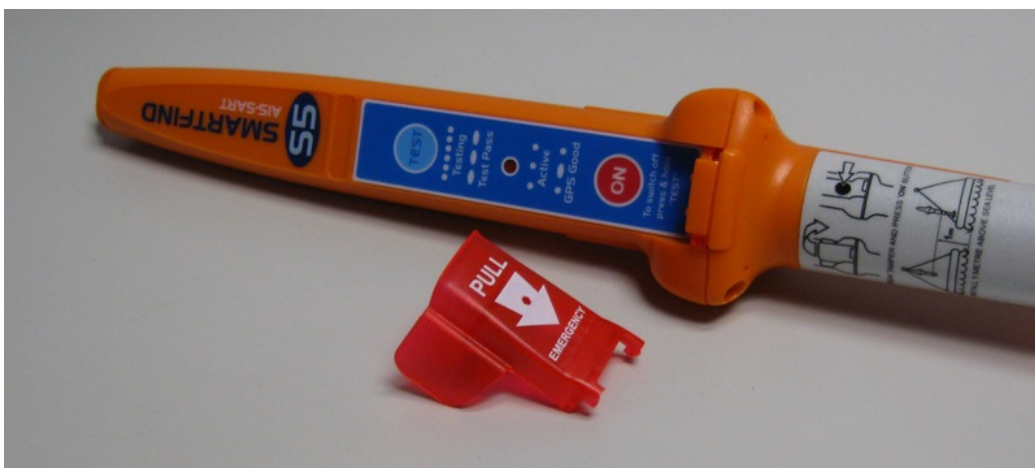
McMurdo Smartfind S5 - frangible tamper cover removed
