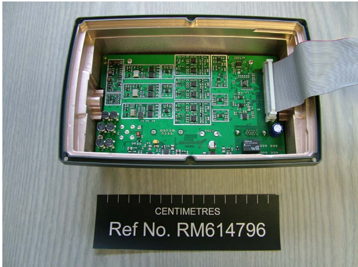
Figure 4: NAV-7 internal view (receivers)
