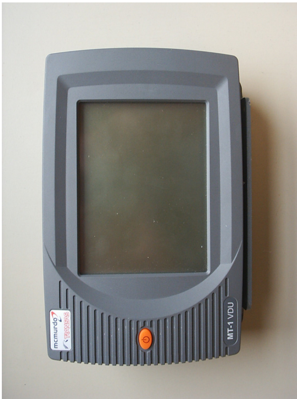
Photograph 2: MT-1 VDU display and control unit
