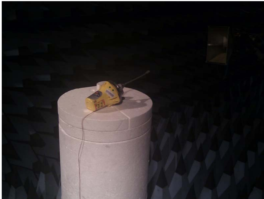
EUT with internal GPS patch antenna facing GPS transmitting antenna (right)
