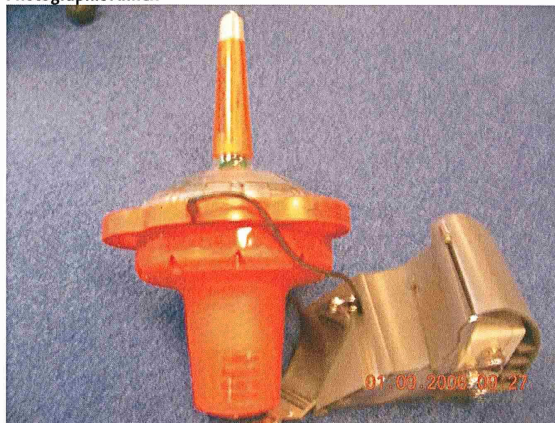
The C1 EPIRB/S-VDR capsule and release bracket.
