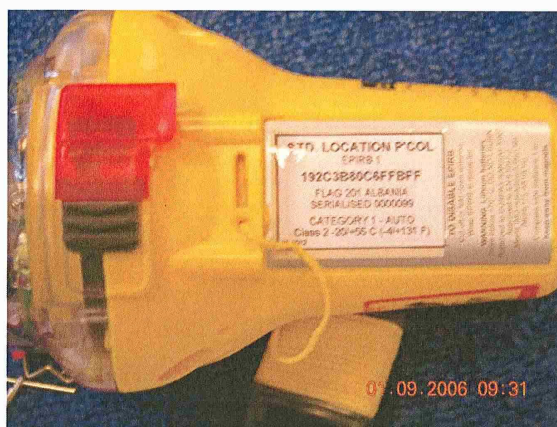
The G5 EPIRB beacon, rear view showing identity label.
