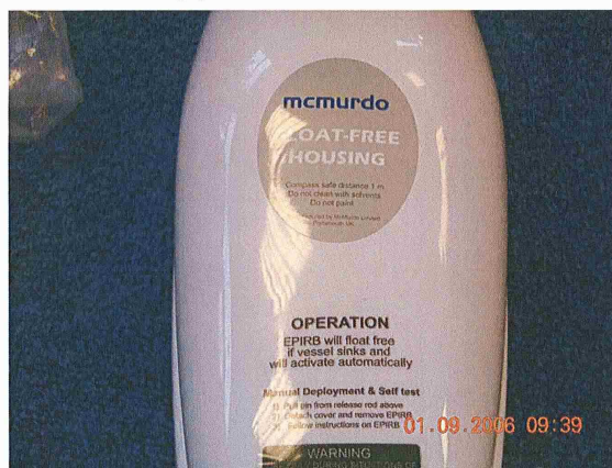
The G5 Float-Free housing, top view showing identity and instruction labels.
