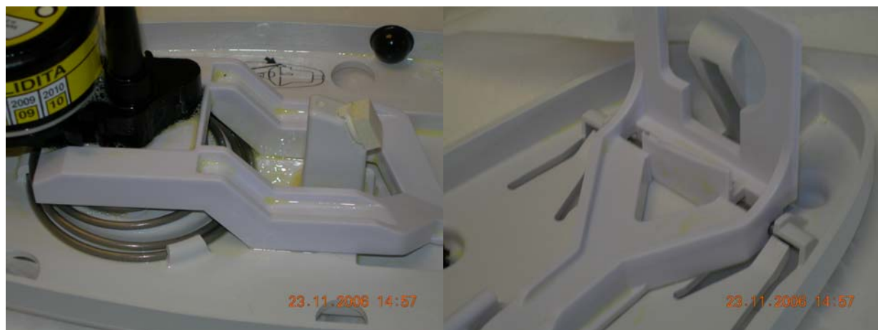
Close-ups of HRU assembly (partially cleaned) and pivot end of cradle lever arm
