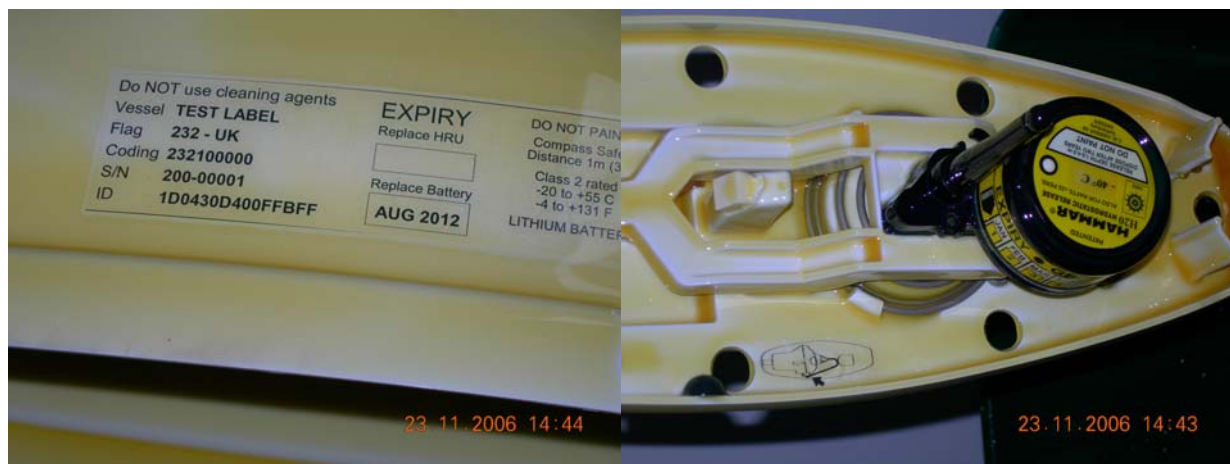
The G5/E5 Float-Free Housing – coding and identity label and interior showing HRU release assembly.
