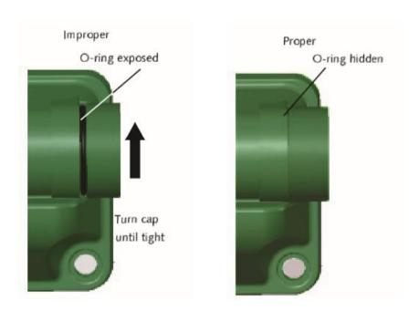
If the O-ring is not properly compressed by the cap, water leakage and damage may occur.
