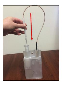
3. Push pin down into the plunger firmly until it clicks into place. Then push the plunger down to arm and lock the sensor.
