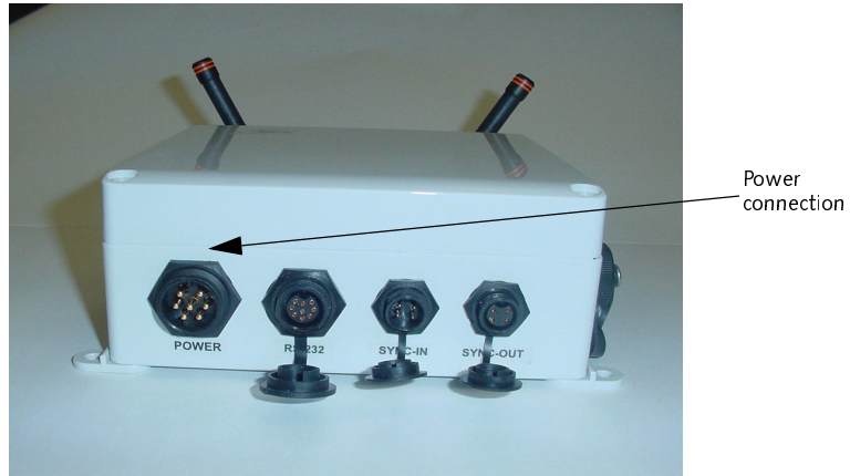
Figure 3-1 Signpost power connection
