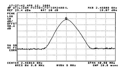
Spurious Emissions, Conducted Test Requirement: 15.247(c)
