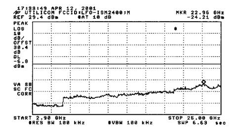
Power Spectral Density Test Requirement: 15.247(d)
