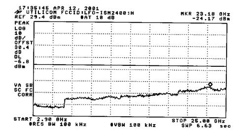
15.247(c): Spurious Emissions, Conducted, HIGH Channel
