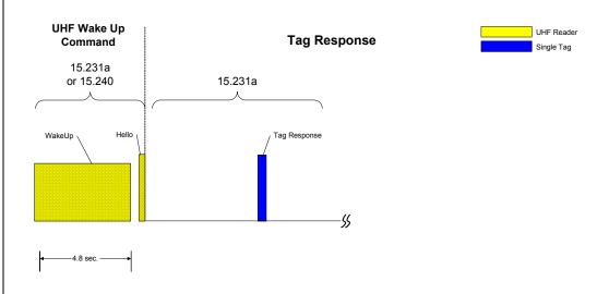
**Mobile (SMR) Reader.** The Wakeup command from a Mobile SMR UHF Reader is comprised of a continuous 31.25 kHz FSK modulated signal on a 433.92 MHz carrier for 2.4 seconds followed by a silent period and a Hello command. The entire signal lasts for less than 5 seconds in compliance with the limit set forth in Section 15.231(a). A timing diagram is depicted below.
