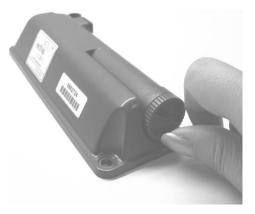
2. Remove the discharged battery from its compartment.
