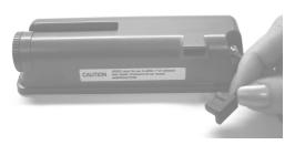
4. Insert Savi Tag Write Cable STA-1030 or Savi Tag Write Cable Adapter STA-1031, with the LED up, into the tag commissioning port. Start the tag commissioning application. The LED is lit when the application writes data to the tag.
