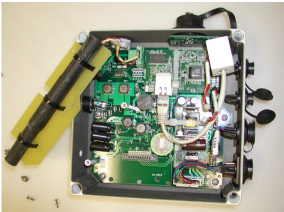
Device with internal ferrite antenna
