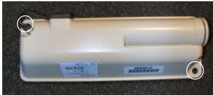
Figure 2-7 SaviTag ST-654 mounting holes
