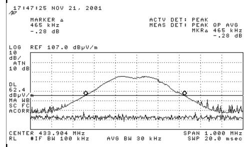
**Duty cycle:** There are never more than two transmissions in a 125mS period. The maximum on time was 4.9mS for a single transmission. The average correction factor to be aplied to peak readings is, therefore, the maximum of -20dB.
