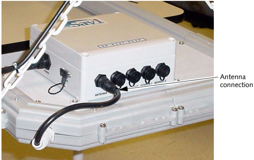
Figure 2-5 Model SP-600-201 or SP-600-211 Signpost Antenna Connection
