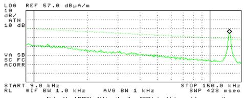
Note: Used RBW = 1kHz rather than 200Hz to obtain a quicker sweep time
