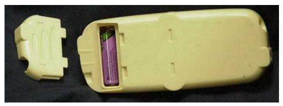
2. Remove the discharged battery from its compartment.
