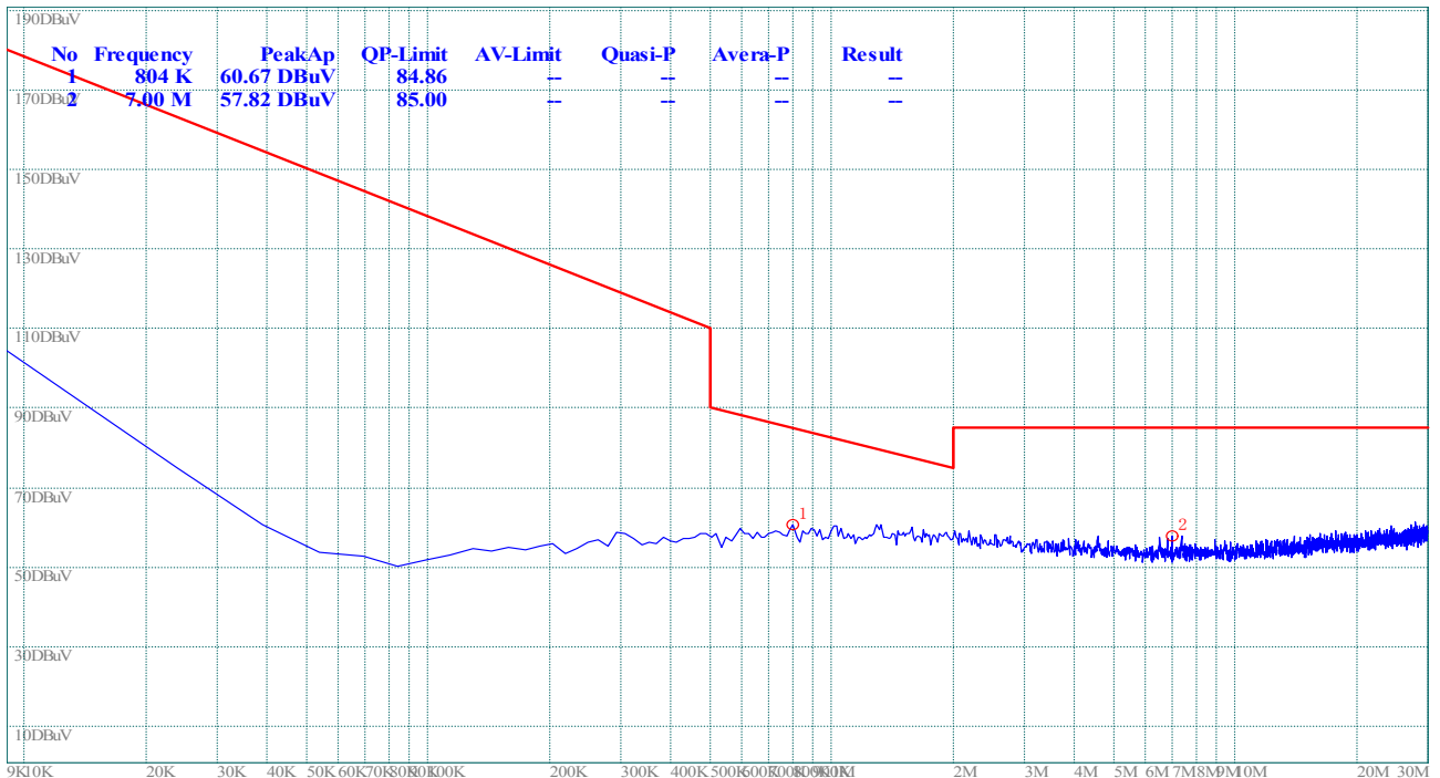
(Plot B.0: 9kHz to 30MHz @ 8-DPSK, channel 39)
