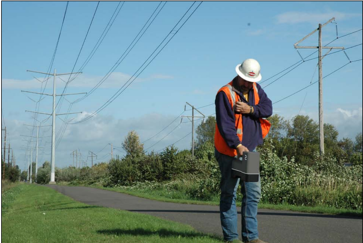
Locating in High-Interference Area with the F2 Receiver
