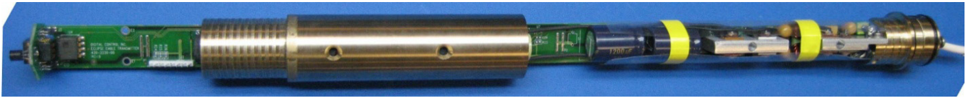
Board with heat sink tube showing and power base attached
