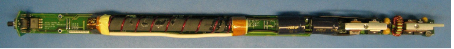
Circuit board top, base and heat sink tube removed
