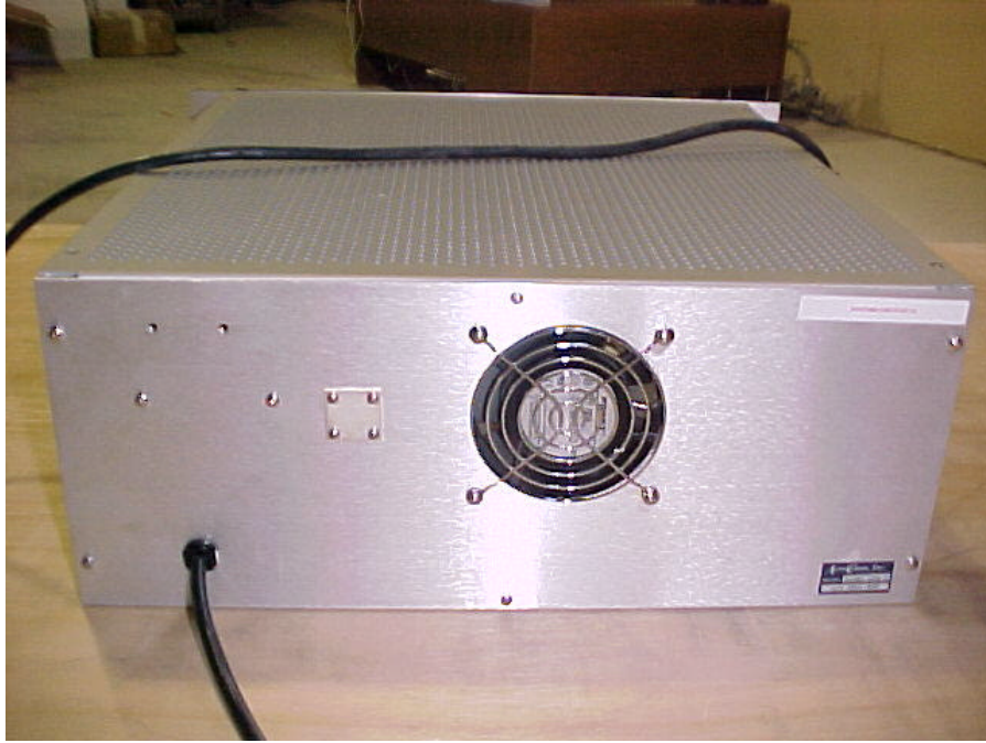
PHOTOGRAPH OF EUT – Donor Unit Power Outlet With A Line Filter
